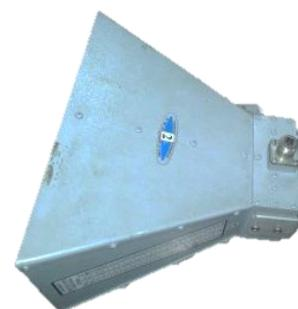
Fig 7. Horn Antenna
