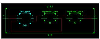
Fig.16: RTL Schematic of Proposed D-FF using Reversible Logic
