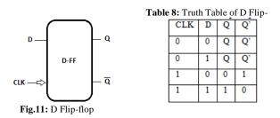
In general D Flip flop is used to design shift registers. The block diagram of D-FF and its truth table is drawn in the above figures. The characteristic equation of D-FF is
