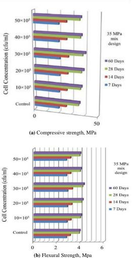
Fig. 2: Impact of various microbial concentration in enhancing the compressive and flexural strength of concrete based on  $f_c = 35$  MPa mix design [Andalib et al 2016].
