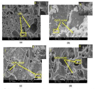
**Fig. 5:** SEM of (a) Specimens without bacteria submerged in water; (b) Specimens with bacteria in aggregates and mixing water; (c) Specimens with bacteria in mixing water; (d) Specimens cast with aggregates filled with bacteria sediment submerged in Urea-CaCl<sub>2</sub>.
