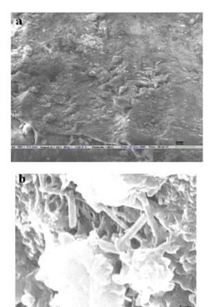
**Fig. 4:** SEM showing bacterial calcite precipitation in cracks of concrete: (a) sample of cement mortar without bacteria, (b) sample taken nearby to surface of healed crack, displaying calcite crystals with rod formed Bacillus sp. CT-5.
