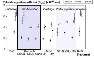
**Fig. 3:** Chloride migration coefficients, Dnssm, for distinctive grades of applied with different kinds of surface treatments.
