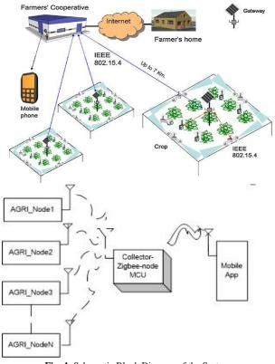
Fig. 4: Schematic Block Diagram of the System.
