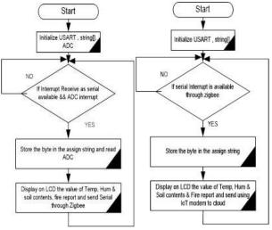
Fig. 9: A) Flow Chart of One Node Using Zigbee B) Flow Chart of Collector-ZigBee-Node MCU and Cloud Server/Mobile App.
