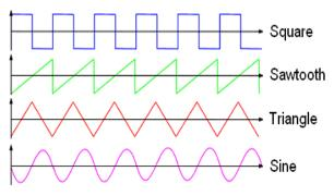
Fig. 3: AF Waveforms [4].
