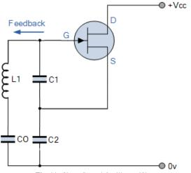
Fig. 11: Clapp Crystal Oscillators [8].
