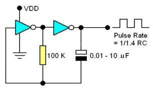
Fig. 4: Diagram of TTL Oscillator [5].
