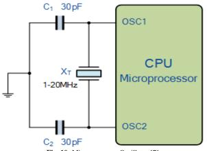
Fig. 10: Microprocessor Oscillator [7].
