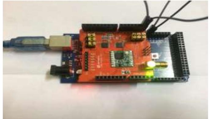
Fig. 4: DRAGINO Shield with Arduino MEGA 2560.
