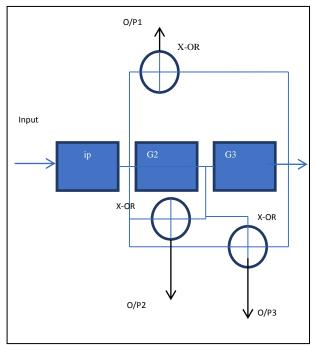
Fig. 4: The Structure of Convolution Coder.
