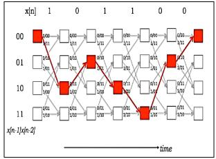
Fig. 6: The Minimum Hamming Distance to Derive the Transmitted Stream in Viterbi Decoder.
