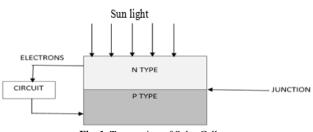
Fig. 1. Transection of Solar Cell
