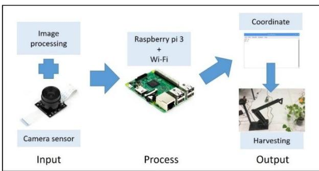
Fig. 1: The Overall Project Architecture.
