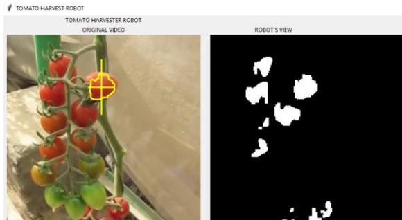
Fig. 4: Image Processing Module.
