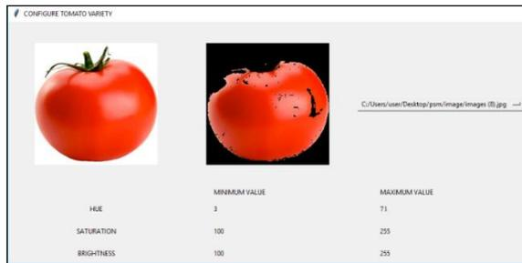
Fig. 5: One of the Process of Training in Image Recognizing Module.
