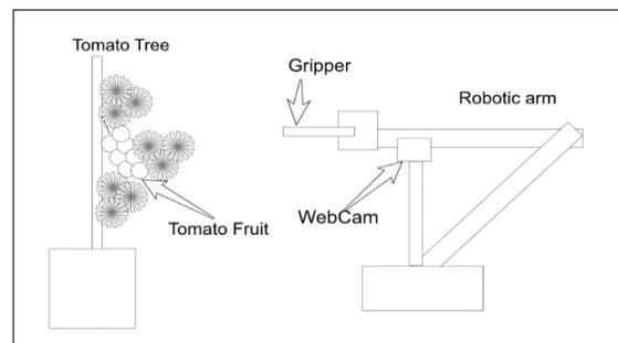
Fig. 3: Tomato Harvester Robotic Arm Prototype Layout.
