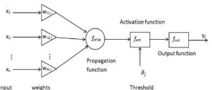
Fig.3: Artificial Neural Network with Activation Function.
