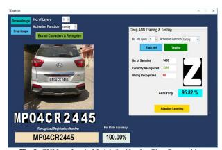
$\textbf{Fig. 8:} \ \textbf{GUI} \ \textbf{Interface in Matlab for Number Plate Recognition}.$
