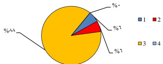
Fig. 7. Percentage . of individual indicators of the condition of contact wires “Wln” in relation to the number of devices (1- $0.00 \leq W_{ln} \leq 0.25$ ; 2- $0.25 < W_{ln} \leq 0.83$ ; 3- $0.83 < W_{ln} \leq 0.99$ ; 4- $W_{ln}=1$ )
