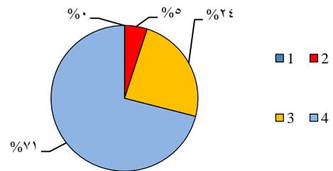
Fig. 6. Percentage of individual indicators of the condition of contact wires “Wdjp” in relation to the number of devices (1- $W_{djp}=1$ ; 2- $0.83 < W_{djp} \leq 0.99$ ; 3- $0.00 \leq W_{djp} \leq 0.25$ ; 4- $0.25 < W_{djp} \leq 0.83$ )
