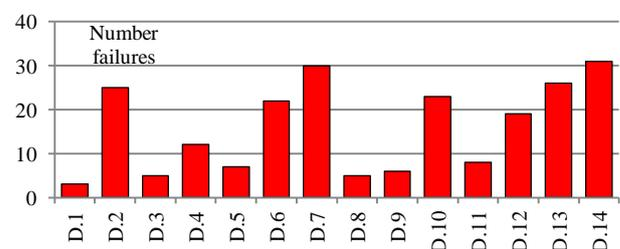
**Fig. 2:** Number of failures from Group I in the analyzed districts of the 3 kV DC power supply network (D.1-District 1, etc.)
