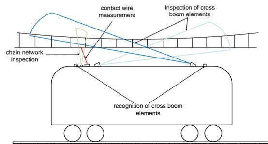
**Fig. 4.** Distribution of inspection systems in a diagnostic car
