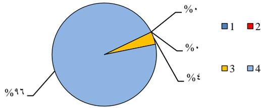
**Fig. 8.** Percentage of individual indicators of the condition of contact wires “Wk” in relation to the number of devices (1- $0.00 \leq Wk \leq 0.25$ ; 2-  $0.25 < Wk \leq 0.83$ ; 3-  $0.83 < Wk \leq 0.99$ )
