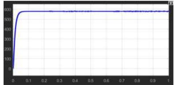
Fig.2: Output Voltage of Constant DC Source fed Zeta Converter
