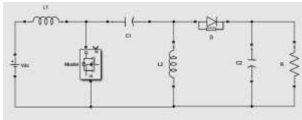
Fig.1: Equivalent Circuit diagram of Zeta Converter
