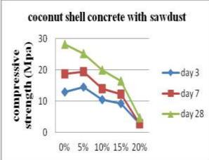
Figure 2: Comparison of CC and CSC with percentage of sawdust
