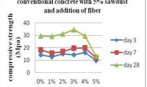
Figure 3: Comparison of CCS and CCQ for 5% sawdust with addition % of fibre
