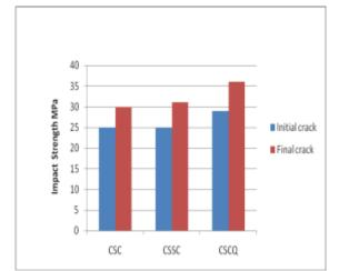
Figure 10: Bar chart of CSC, CSSC, CSCQ without addition of fibre
