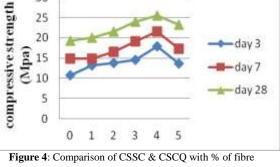
The Table 4 and Figure 4 shows that CSSC has a greater value of 33.32 Mpa at 2% of fibre while CSCQ has 25.50 Mpa at 4% of fibre. In case of coconut shell concrete CSSC shows good improvement when fibre is added to it in comparison to 0% fibre.
