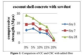
The content of sawdust replaced in controlled and coconut shell concrete is in the percentage of 5%, 10%, 15% and 20% to the volume of fine aggregate. the results were shown in Table 2 and the comparison for CC and CCS in made in Figure 2.
