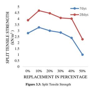
Splitting tensile strength is maximum for 10%. Other moulds showed decrease in strength.
