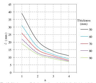
**Fig.13:** Displacement ( $\delta$ ) for hyperbolic paraboloid shell of height 1.818 m
