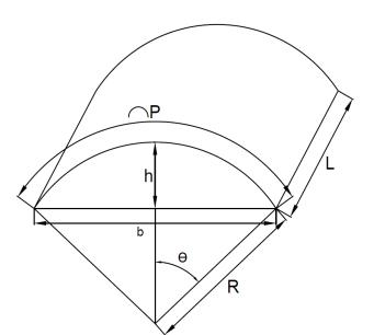
**Fig.1**: Isometric view of cylindrical shell roof (CS).  $h = \text{Height}; R = \text{Radius}; \\ \theta = \text{Semi-central angle}; L = \text{Length}; b = \text{bay width}; P = \text{Circumference}$
