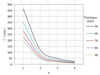
Fig.9: Displacement ( $\delta$ ) for cylindrical shell of height 1.67 m
