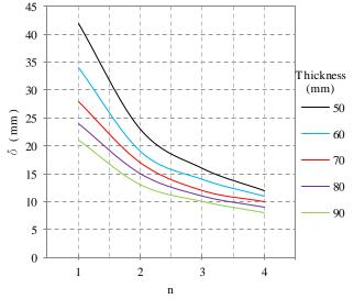
Fig.14: Displacement ( $\delta$ ) for hyperbolic praboloid shell of height 1.67 m
