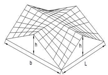
**Fig.2:** Isometric view of hyperbolic paraboloid shell roof (HPS). h = Height; L = Length; b = bay width
