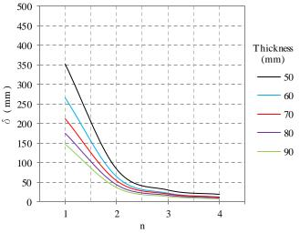
Fig.6: Displacement ( $\delta$ ) for cylindrical shell of height 2.22 m
