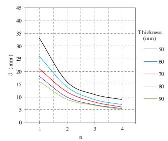
**Fig.11**: Displacement ( $\delta$ ) for hyperbolic paraboloid shell of height 2.22 m
