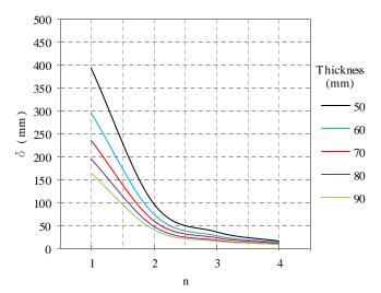
**Fig.7**: Displacement ( $\delta$ ) for cylindrical shell of height 2 m
