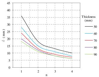
**Fig.12:** Displacement  $(\delta)$  for hyperbolic paraboloid shell of height 2 m
