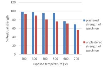
Fig 5: Residual Strength of concrete cube coated with PC mortar against Exposure Temperature.
