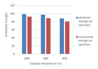
Fig. 2: Residual strength of concrete cube coated with SC mortar against Exposure Temperature
