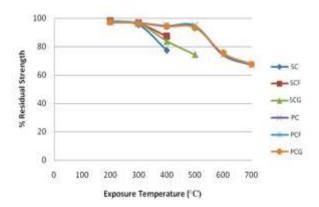
Fig 8: Residual strength of concrete cubes coated with various mortar subjected to elevated temperatures
