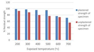
Fig. 6: Residual Strength of concrete cubes coated with PCF mortar against Exposure Temperature
