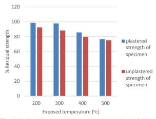
Fig. 4: Residual Strength of concrete cubes coated with SCG mortar against Exposure Temperature
