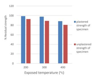
Fig. 3: Residual strength of concrete cube coated with SCF mortar against Exposure Temperature
