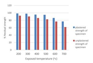
Fig. 7: Residual Strength of concrete cubes coated with PCG mortar against Exposure Temperature
