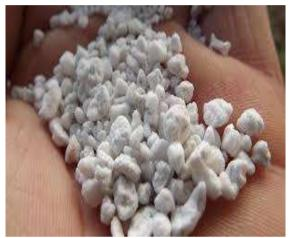
Fig. 1: Expanded perlite aggregate
