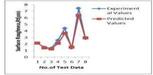
Fig 5: Predicted and Experimental values obtained for Rt (test data)
