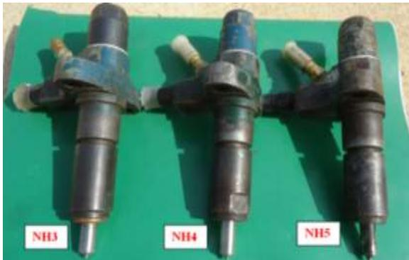
Fig.2: Photographic view of 3, 4 and 5 whole nozzle fuel injectors
