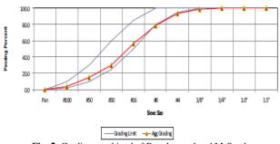
Fig. 5: Grading combined of Bangka sand and M-Sand.
