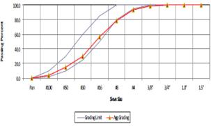
Fig. 3: Grading Material of Bangka Sand / Belitung.
