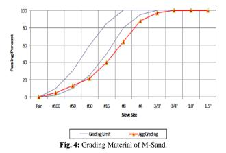
From the picture above shows that a 3/4 sieve of 100% means msand is finer than bangka sand which means better mixing of concrete because the air cavity in concrete will be filled with ash so that the mixture is more solid than pure bangka sand. River sand was replaced by manufactured sand (M-sand) at replacement levels of 20,40,60,80 and 100% [12].
