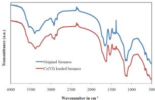
Fig. 3: FTIR Analysis of the Original and Cr (VI) Loaded Microalgae Biomass.
