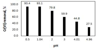
**Fig. 5:** Effect of Initial Ph on the Cr (VI) Removal. (Conditions: Initial Cr(VI) Conc., 10 Mg/L; Solid-Liquid Ratio, 10 %(W/V); Contact Time, 150 Min; Temp., 30 Oc; Particle Size, -75+45 µm; Stirring Speed, 200 Rpm)
