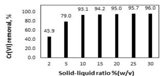
**Fig. 6:** Effect of Adsorbent Dose on the Cr (VI) Removal. (Conditions: Initial Cr(VI) Conc., 10 Mg/L; Initial Ph, 1.0; Contact Time, 150 Min; Temp., 30 Oc; Particle Size, -75+45 μm; Stirring Speed, 200 Rpm).
