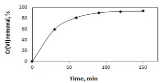
**Fig. 4:** Effect of Contact Time on the Cr (VI) Removal. (Conditions: Initial Cr(VI) Conc., 10 Mg/L; Solid-Liquid Ratio, 10 %(W/V); Initial Ph, 1.0; Temp., 30 Oc; Particle Size, -75+45 μm; Stirring Speed, 200 Rpm).
