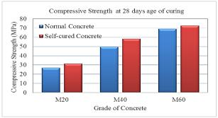
Fig. 2: Compressive Strength Properties of Normal and Self-Curing Concrete Mixes at 28 Days Age of Curing.
