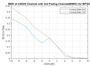
Fig. 16: BER Vs SNR for BPSK Technique Fig. 16 Gives Variation of BER for Various Values of SNR for 3/4 and 1/2 Coding Rate.
