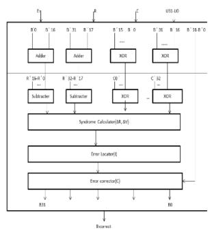
Fig. 3.7: Block Diagram of Decoder.
