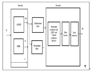
Fig. 3.1: Fault Tolarent Memory Block.
