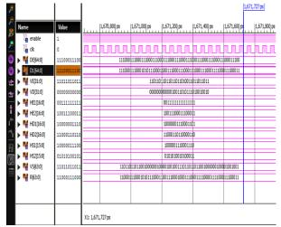
Fig. 4.3: Simulation Results of 64 Bit Data Split Into 4 Symbols
