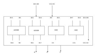
Fig. 3.4: Block Diagram of Encoder.
