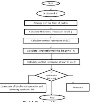
Fig. 3.3: Flowchart of Decoder.
