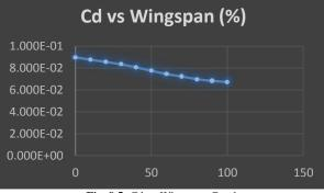
Fig. 8.5: Cd vs Wingspan Graph.
