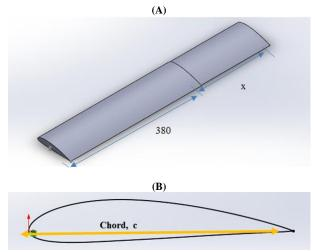
Fig. 3.4: Half Wing Dimension of NACA 4415 (AoA =  $1^{\circ}$ ).
