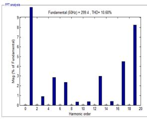
Fig. 7: C): FFT Analysis of 7-Level Inverter with POD-SPWM.
