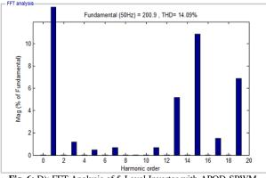
Fig. 6: D): FFT Analysis of 5-Level Inverter with APOD-SPWM.
