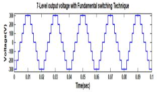
Fig. 8: C): 7-Level Output Phase Voltage Profile Using Bee Algorithm.
