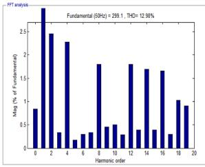
Fig. 7: B): FFT Analysis of 7-Level Inverter with PD-SPWM.
