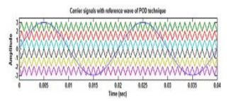
Fig. 3: B): Comparison of Reference and Carrier Signals of POD for 7-Level CHB Inverter.
