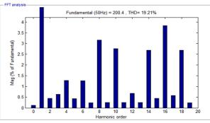
Fig. 6: B): FFT Analysis of 5-Level Inverter with PD-SPWM.
