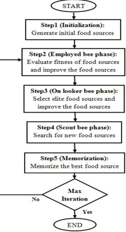
Fig. 5: Flowchart of Bee Algorithm.
