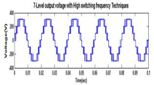
Fig. 7: A): 7-Level Output Phase Voltages of CHMLI Using PD, POD and APOD Techniques.
