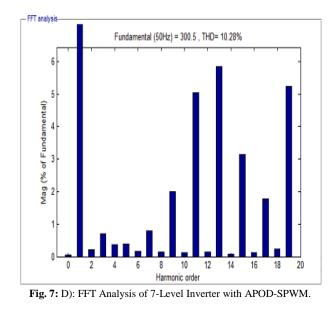
The THD's of 7-level CHB inverter with PD-SPWM technique is 12.98%, POD-SPWM technique is 10.60% and APOD-SPWM is 10.28%.
