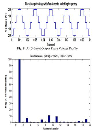
Fig. 8: B): FFT of 5-Level CHMLI Using Bee Algorithm.
