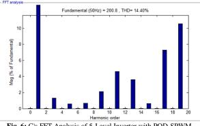
Fig. 6: C): FFT Analysis of 5-Level Inverter with POD-SPWM.
