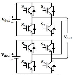
Fig. 1: 5-Level CHB Inverter Circuit
