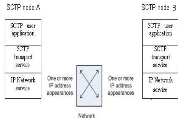
Fig. 2: SCTP Association between two end nodes
