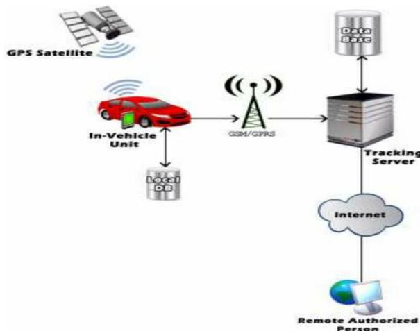
Fig. 1: Vehicle Tracking System.
