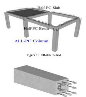
Figure 2: Hollow-PC Column
