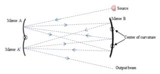
Figure 1: Diagram of White cell principle.
