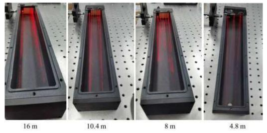
Figure 3: Patterns of different path lengths of the NDIR gas cell.
