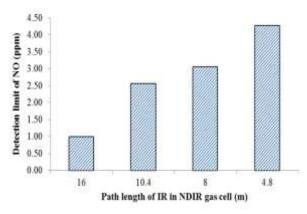
Figure 5: Relationship between detection limit of NO and optical path length of the gas cell.
