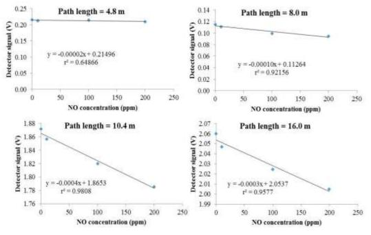
Figure 4: Variations of detector signals associated with NO concentrations and optical path lengths.
