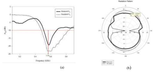
Figure 3: (a) Comparison between measured and simulated of the return loss,  $S_{11}$  of the microstrip; (b) Comparison of 2-dimensional radiation pattern between the measured and simulated results antenna.
