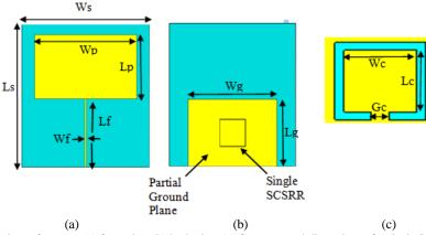
Figure 1: Geometry and dimensions of antenna (a) front view (b) back view (c) Geometry and dimensions of a single Slotted Complementary Split Ring Resonator (SCSRR)
