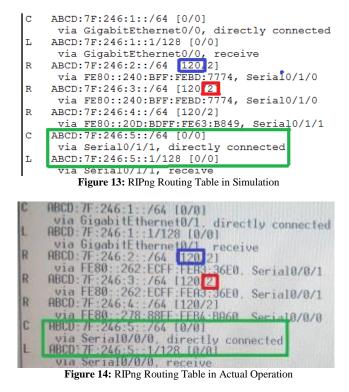
Results in IPv6 network for both simulation and actual operation in EIGRPv6 are the same in directly connected networks and administrative distance as shown in the green and blue highlighted data respectively; however, the highlighted information in red shows the differences in metric data.
