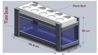
Fig. 2: Our Aquaponics Design using Solidworks.
