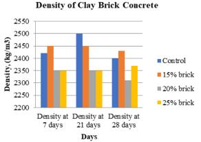
Fig 3: Density of hardened clay brick concrete
