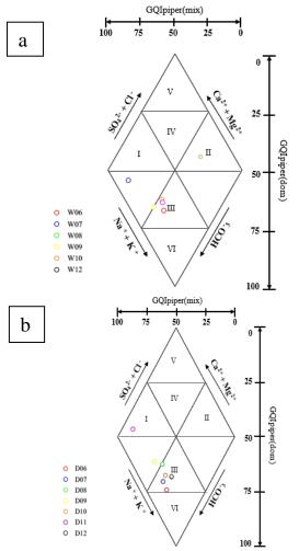
**Fig. 1:** Piper diagram of groundwater samples collected during wet period (a) and dry period (b)
