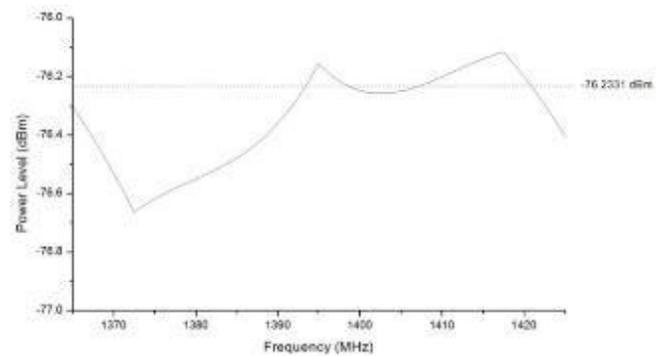
Fig. 6: Average RFI level in HI suggested minimum bandwidth
