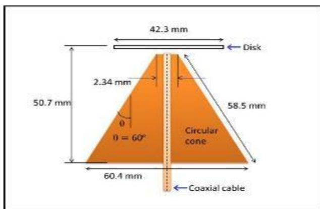
Fig. 1: The schematic geometry of the discone antenna.
