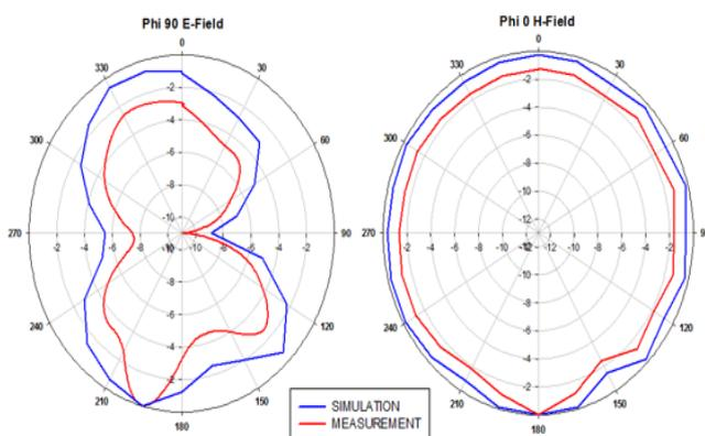
Fig. 5: Polar plot for proposed antenna (a) Phi 90 (b) Phi 0.
