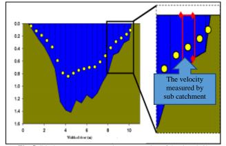
Fig. 5: Discharge measurement by cross section of the river [10]
