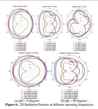
The far field radiation patterns of the antenna at different resonant frequencies are given in Fig 6. At lower operating band antenna is showing omni directional pattern in H-field and at higher operating band antenna is showing quasi omni directional pattern.
