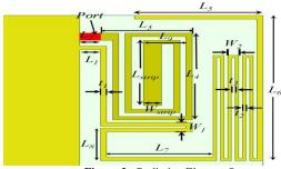
Figure 2.: Radiating Element Structure
