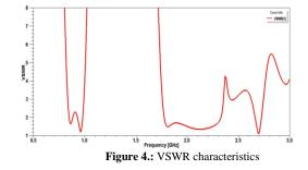
The operating bands and their bandwidth are clearly mentioned in the table 2. The voltage standing wave ratio is one of the important parameter to analyze the bandwidth of the antenna. Ideally it should be one and practically 2:1 ratio should be maintained. Fig 4 shows the VSWR of 2:1 ratio at operating bands and table 3 gives the VSWR operating bands and corresponding bandwidth.
