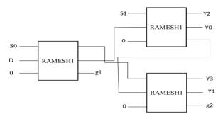
Figure 21: Block Diagram of 1:4 Demultiplexer using RAMESH-1 Reversible Logic Gate.
