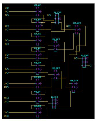
Figure 25: Schematic Diagram of 16:1 Multiplexer using QCA Reversible Logic Gate.
