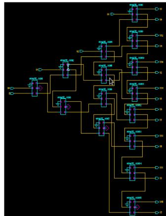
Figure 28: Schematic Diagram of 1:16 Demultiplexer using RAMESH Reversible Logic Gate.
