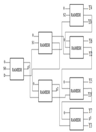
Figure 18: Block Diagram of 1:8 Demultiplexer using RAMESH Reversible Logic Gate.
