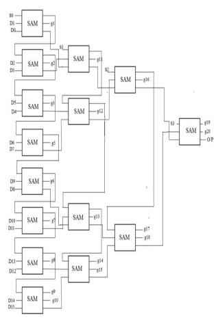
Figure 12: Block Diagram of 16:1 Multiplexer using SAM Reversible Logic Gate.
