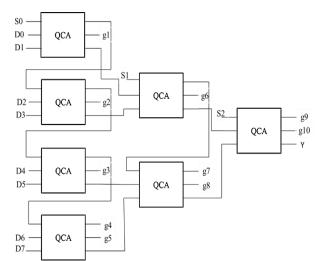
Figure 7: Block Diagram of 8:1 Multiplexer using QCA Reversible Logic Gate.
