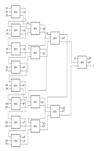
Figure 8: Block Diagram of 16:1 Multiplexer using QCA Reversible Logic Gate.
