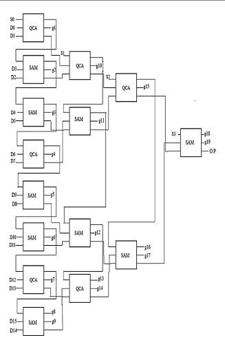
Figure 15: Block Diagram of 16:1 Multiplexer using QCA and SAM Reversible Logic Gates.
