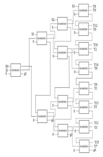
Figure 23: Block Diagram of 1:16 Demultiplexer using RAMESH-1 Reversible Logic Gate.
