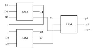
Figure 10: Block Diagram of 4:1 Multiplexer using SAM Reversible Logic Gate.
