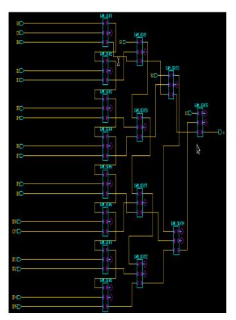
Figure 26: Schematic Diagram of 16:1 Multiplexer using SAM Reversible Logic Gate.
