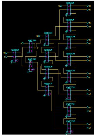
Figure 29: Schematic Diagram of 1:16 Demultiplexer using RAMESH-1 Reversible Logic Gate.
