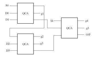
Figure 6: Block Diagram of 4:1 Multiplexer using QCA Reversible Logic Gate.
