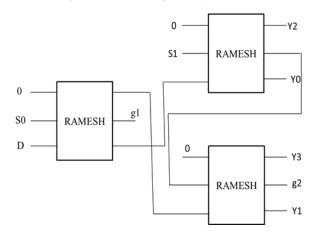
Figure 17: Block Diagram of 1:4 Demultiplexer using RAMESH Reversible Logic Gate.
