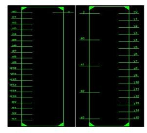
Figure 24: Black Box View of 16:1 Multiplexer using QCA, SAM, and QCA & SAM and 1:16 Demultiplexer using RAMESH and RAMESH-1 Reversible Logic Gates.
