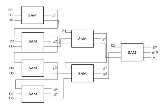
Figure 11: Block Diagram of 8:1 Multiplexer using SAM Reversible Logic Gate.
