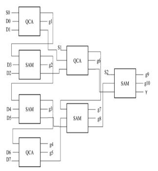
Figure 14: Block Diagram of 8:1 Multiplexer using QCA and SAM Reversible Logic Gates.
