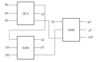
Figure 13: Block Diagram of 4:1 Multiplexer using QCA and SAM Reversible Logic Gates.
