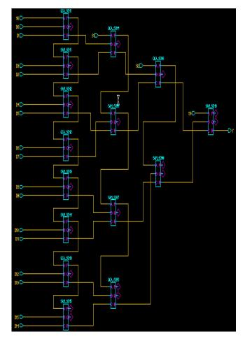
Figure 27: Schematic Diagram of 16:1 Multiplexer using QCA and SAM Reversible Logic Gates.
