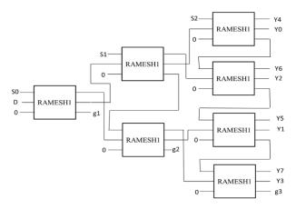
Figure 22: Block Diagram of 1:8 Demultiplexer using RAMESH-1 Reversible Logic Gate.
