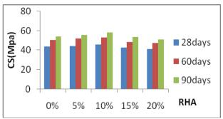
Fig. 3: RHA Concrete cured in 3% Magnesium Sulfate Solution (MgSO<sub>4</sub>)
