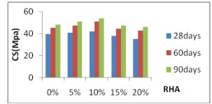
Fig. 4: RHA Concrete cured in 5% Magnesium Sulfate Solution (MgSO<sub>4</sub>)
