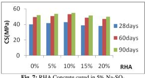
Fig. 7: RHA Concrete cured in 5% Na<sub>2</sub>SO<sub>4</sub>
