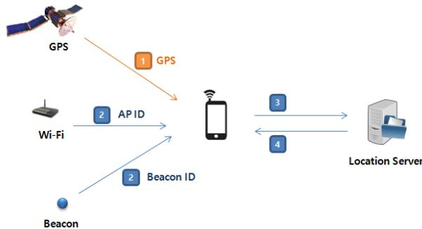
Figure 1.:Concept of mixed positioning
