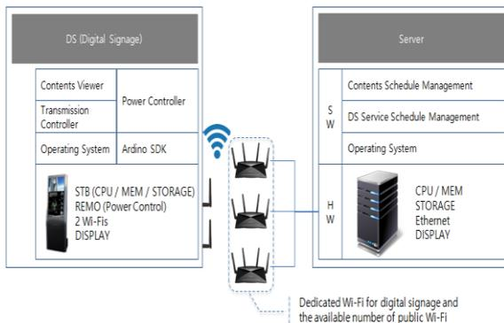
Figure 2.:Configuration diagram of the complete system
