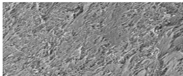
Figure 3: Picture of CNT by SEM
