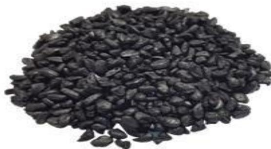
Figure 4: CNT composite pellet
