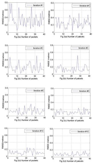
Fig. 2 & Fig. 3 : Variations in the RMSE value of TDOA localization algorithm using RLS (Left side column) and TDOA-DV localization algorithm using RLS (Right side column).
