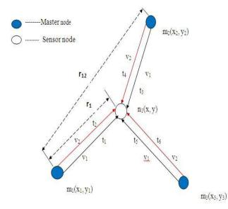
Fig. 1: Schematic of Time Difference of Arrival-Dual Velocity.
