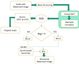
Fig. 5 Proposed Digital Audio Watermark Extracting Algorithm
