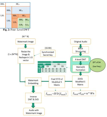
Fig. 3: Proposed Digital Audio Watermark Embedding Algorithm
