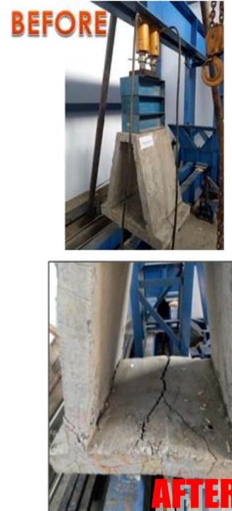
Fig. 4: Precast foundation design and pressure test [1]
