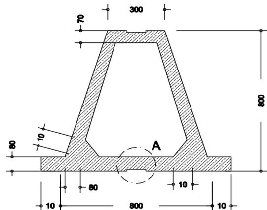
**Fig. 9:** Precast Foundation Design [1],[4]
