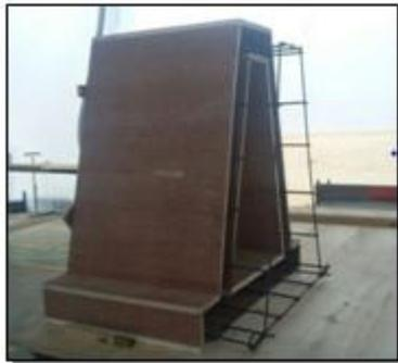
**Fig. 6 :** Formwork precast and wire mesh A model
