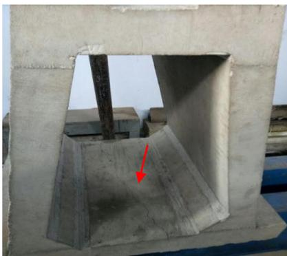
Fig.13: Side wall – bottom crack foundation
