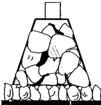
Fig. 2: Typical stone foundation [8]
