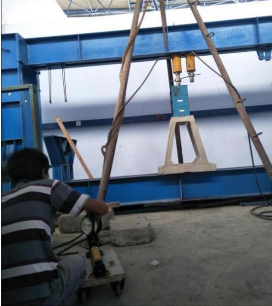
Fig.12: Pressure Test Precast Foundation Models
