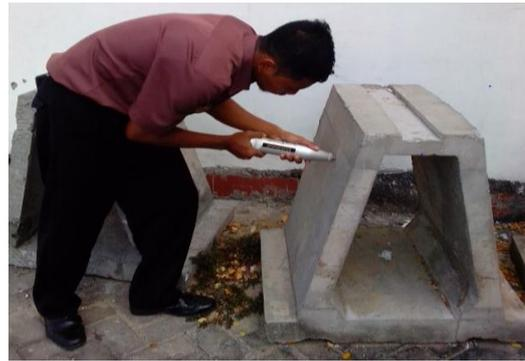
Fig. 14: Pressure Hammer Test Precast Foundation Model
