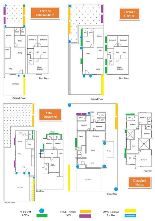
Fig. 4: The Possible Locations for Installing Space Saving Rainwater Harvesting Tanks.
