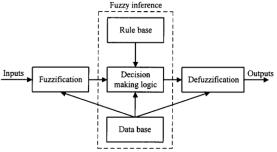
Fig. 1: Represents the block diagram of fuzzy logic
