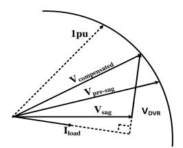
Fig. 7:In-Phase Advanced/Energy Optimization Compensation.
