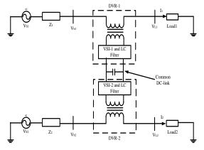
Fig. 8: 2-Lines Inter-Line Dynamic Voltage Restorer (IDVR).
