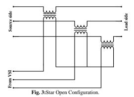
If the upstream transformer is an earthed star-star configuration, then zero sequence voltages must be compensated [29]. For this case, a star-open injection transformer as shown in Fig. 3 is employed [31].
