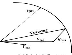
Fig. 6:Pre-Sag Injection/Compensation.
