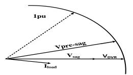
Fig. 5:In-Phase Injection/Compensation.
