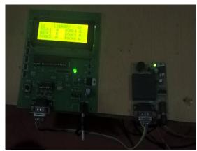
$\textbf{Fig. 6:} \ \textbf{Interfacing of RFID Reader with PIC Microcontroller}$
