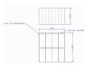
Fig. 2: Dimensions of file rack
