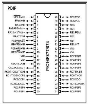
Fig. 4: PIC Microcontroller
