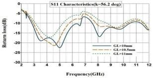
Fig. 7:S<sub>11</sub> Characteristics of Proposed Antenna Varying GL (K=56.2°).
