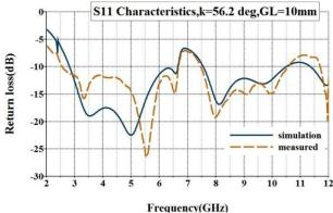
Fig. 6:S<sub>11</sub> Characteristics of Proposed Antenna.
