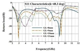
Fig. 10:S<sub>11</sub> Characteristics Antenna Varying GL (K=48.3°) and R=9.3MM.
