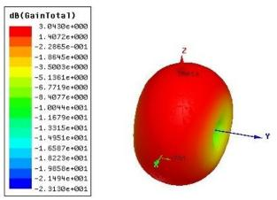
Fig. 17: Gain of the Antenna at 3.3 GHz.
