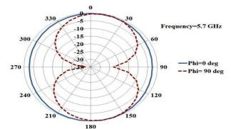
Fig. 12: Radiation Pattern of the Proposed Antenna at 5.7 GHZ.
