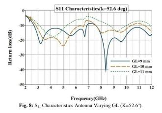
It is observed that when the ground length is maintained proper feed distance (P), bandwidth is significantly improves, when the ground length approaches nearer to radiating patch bandwidth reduces due to interference
