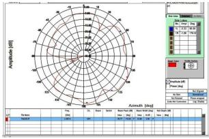
Fig. 13: Tested Radiation Pattern of the Proposed Antenna at 3.3 GHZ and Phi=90 Deg.
