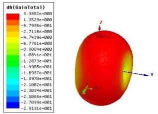
Fig. 18: Gain of the Antenna at 5.7 GHZ.
