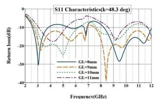
Fig. 9:S<sub>11</sub> Characteristics Antenna Varying GL (K=48.3°) and R=7.3MM.
