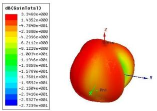
Fig. 19: Gain of the Antenna at 9.1 GHZ.
