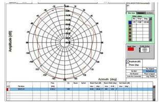
Fig. 14: Tested Radiation Pattern of the Proposed Antenna at 5.7 GHZ and Phi=90 Deg.
