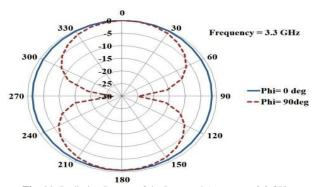
Fig. 11: Radiation Pattern of the Proposed Antenna at 3.3 GHz.
