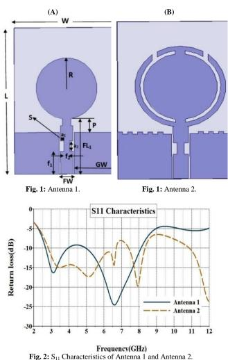
With this modifications Antenna 2 bandwidth (BW) increased to 80.7% from 59.6% of the band 1 as shown in Table 1.But it reduces the bandwidth percentage of band 2.In order to get two wide bands, antenna is proposed with tapered and ridged ground in this paper.
