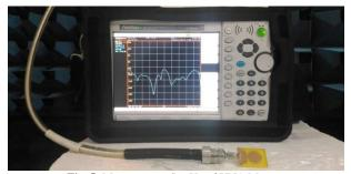
Fig. 5: Measurement Set-Up of VNA Master.
