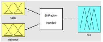
Figure 7: Fuzzy Input and Output Variables for the Fuzzy Skill Predictor
